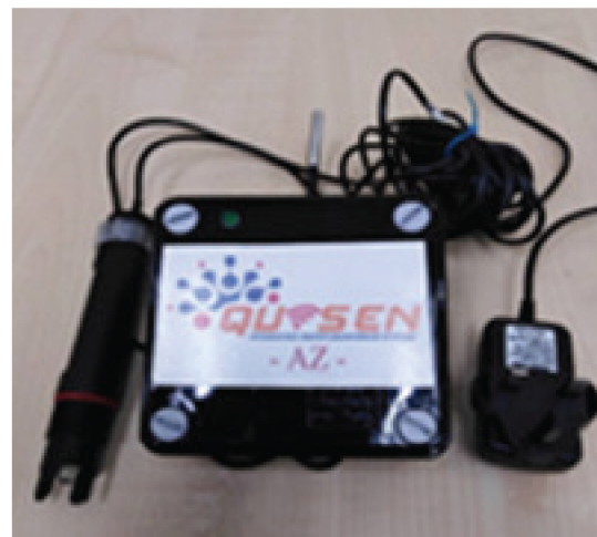
Quasen - Aquaculture Cloud-Based Water Monitoring System
